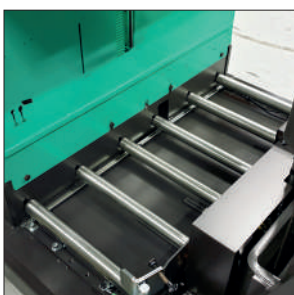
Battery on steel rollers
